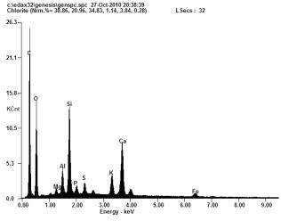
Fig. 12. Chemical analysis of the vermicompost, performed with the application of the EDS microanalyzer.
