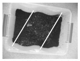
Fig. 8. The result of bioutilization. Visible remains of 1,4-cis polibutadiene rubber in the central part of the sample. On the left and right sides are droppings of *Eisenia faetida* (Photo. M. A. Jóźwiak).
